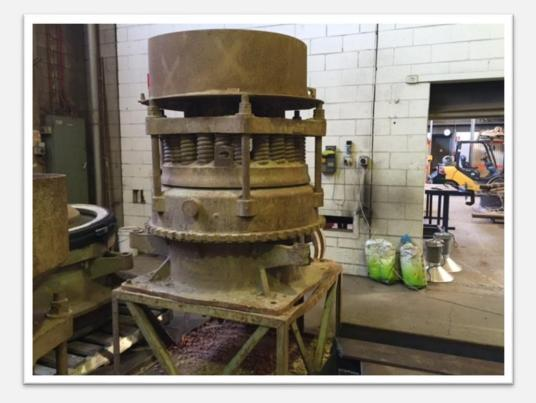
Crusher is currently under repair in the C.P.E. workshop. Will be fitted with new inner & outer bushes and labyrinth seals. Gears are in very good order. Supplied with integral oil pump and external oil tank.
