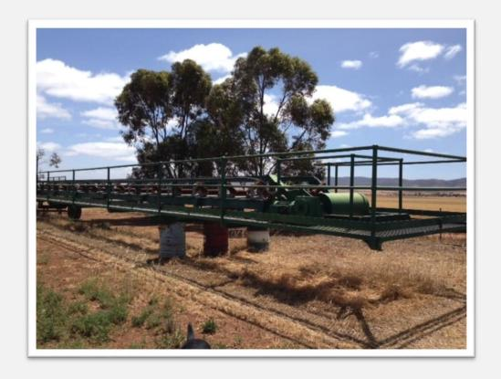
21.4mt x 900mm Conveyor. Includes walkway and SEW 90 degree x 9.2kw drive. New Conveyor Belt is included. Lower stringer fabricated from 180mm UB & upper stringer from 100 UB.
