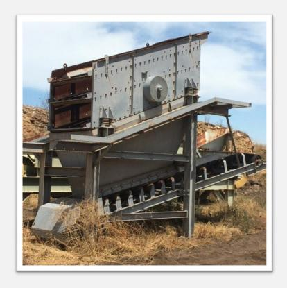
Jaques 12' x 5' T/Deck Screen Module. Includes support fabricated mainly from 200mm UC with walkways and a 6.7mt x 1,050mm under-screen conveyor. Includes electric motor for screen & conveyor drive.
