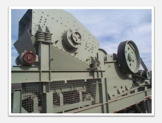
All New Jian-She 600 x 900 Jaw Crusher. Includes 10.5mt x 1.2mt under crusher discharge conveyor, Metro 8' x 4' d/deck scalp screen & 2.4mt x 1,050mm scalps conveyor, all mounted on a h/duty 400mm UB support structure. Also includes all electric motors & conveyor drives.
