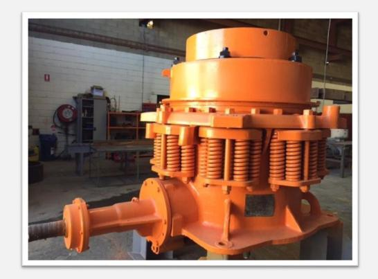
Crusher has been fully repaired in C.P.E.'s workshop. Includes new Socket Liner, Socket Seal Ring, Lock Nut, Lock Nut Cover, Feed Distributor, Feed Plate & reconditioned Head/Shaft and Bowl.
