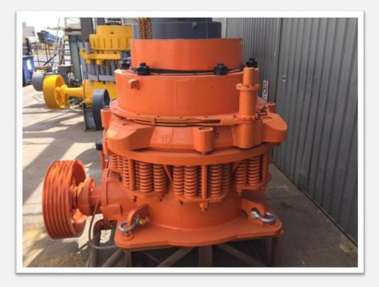
Late model Crusher has been fully repaired in C.P.E. workshop. Includes new Socket Liner & Socket Seal Ring.
