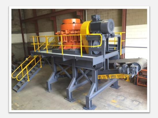
Comprising of a heavy-duty support frame. Crusher can be supplied as a 3ft Std or S/Head configuration and will be fully repaired, includes lube system. Photo for illustration purposes.
